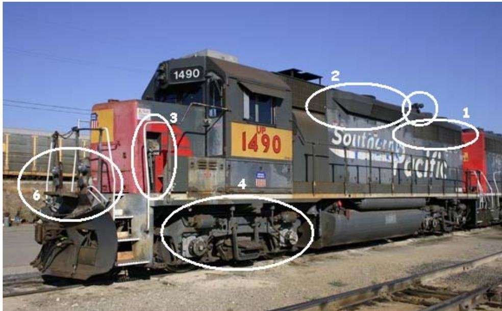
UP patched GP40M-2 #1490, former SP #7120 is a good illustration of the early era GP40-2, although it does not have an SP light array and its bell is below the running board, not roof mounted, and the horn has been moved to the long hood.
